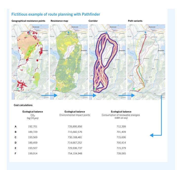
Figure: the five steps of route planning with "Pathfinder", illustrated using a fictitious project: analysis of geographical resistance, creation of a resistance map, definition of suitable corridors, development of route variants and calculation of costs.
